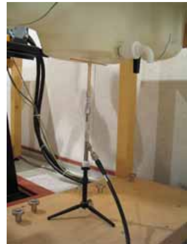
Photo of the dipole Antenna
