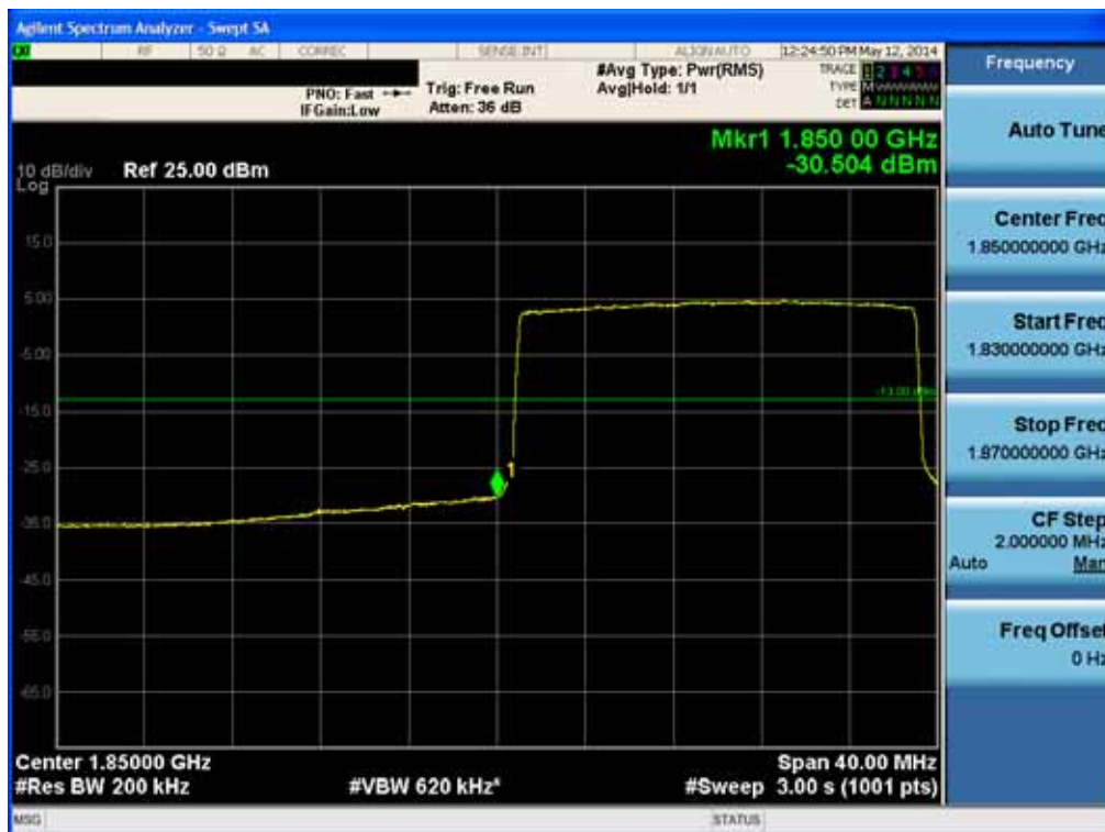
BAND 2. Lower Band Edge Plot (20M BW Ch.18700 QPSK RB 100) -2
