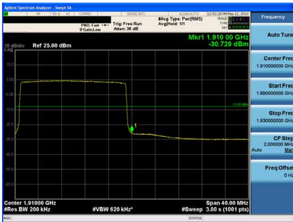
BAND 2. Upper Band Edge Plot (20M BW Ch.19100 QPSK RB 100) -2
