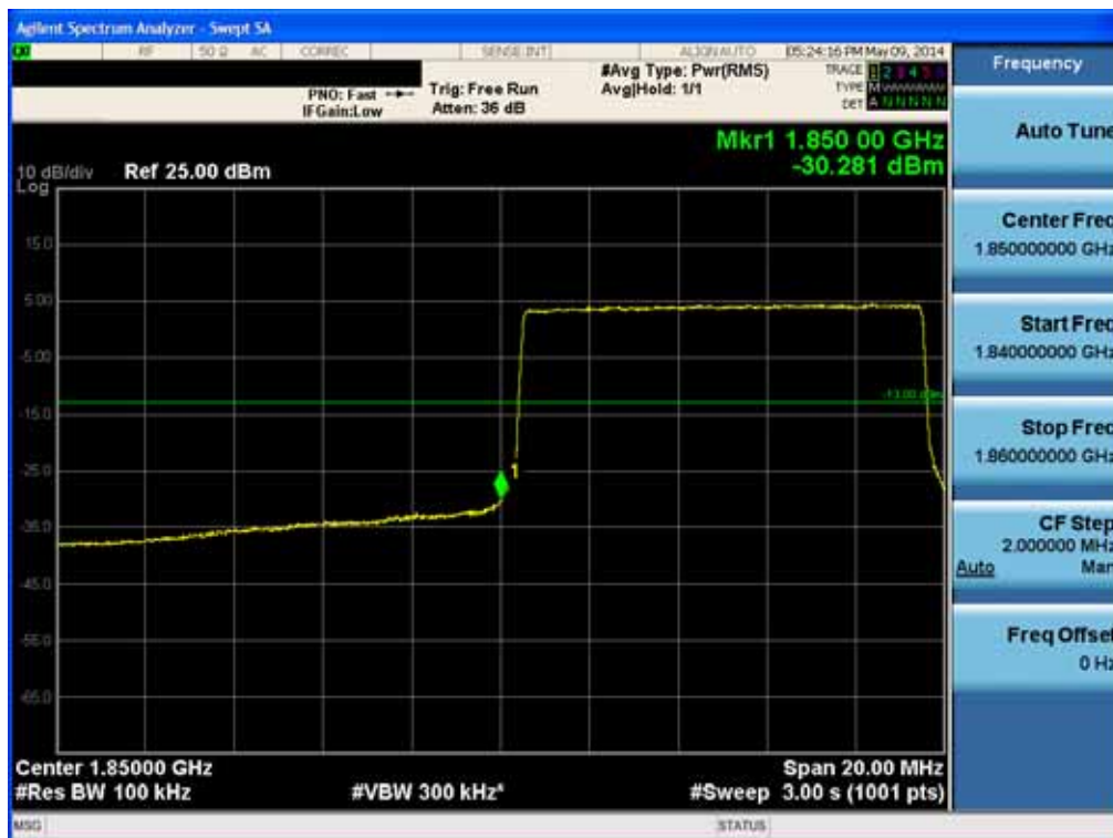
BAND 2. Lower Band Edge Plot (10M BW Ch.18650 QPSK RB 50) -2
