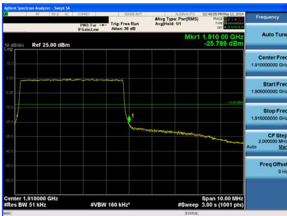
BAND 2. Upper Band Edge Plot (5M BW Ch.19175 QPSK RB 25) -2
