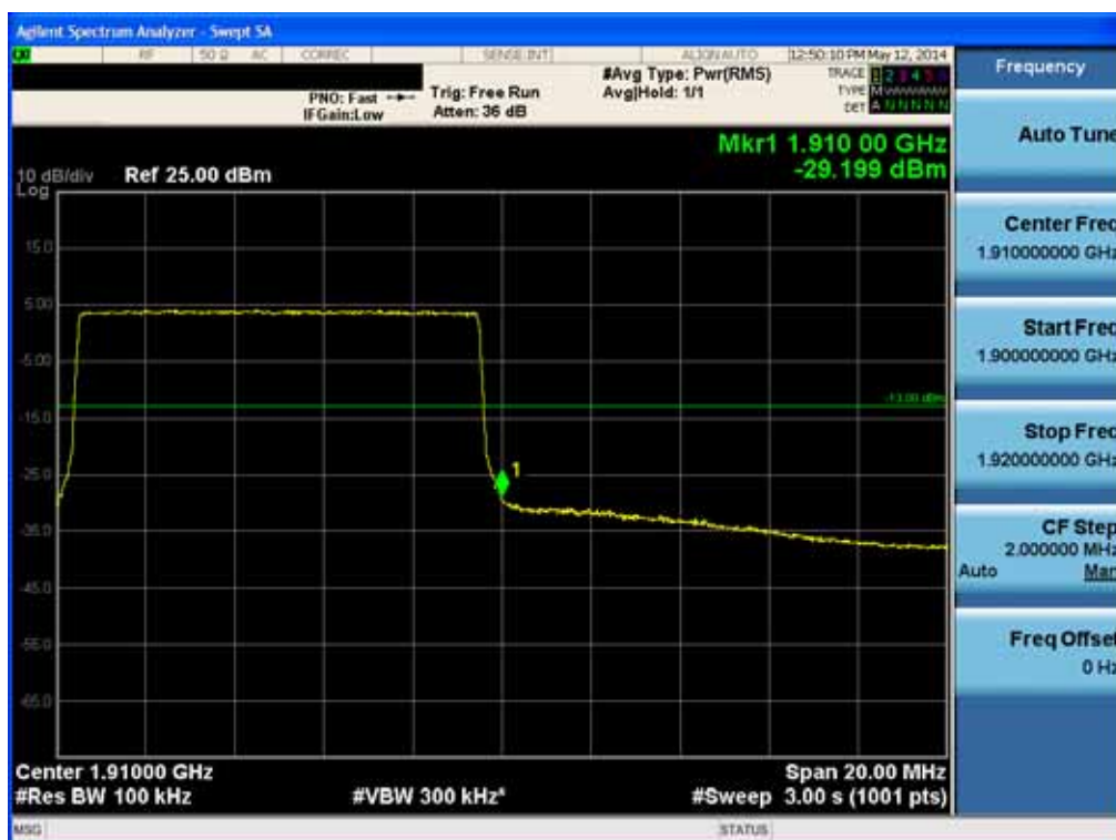
BAND 2. Upper Band Edge Plot (10M BW Ch.19150 QPSK RB 50) -2
