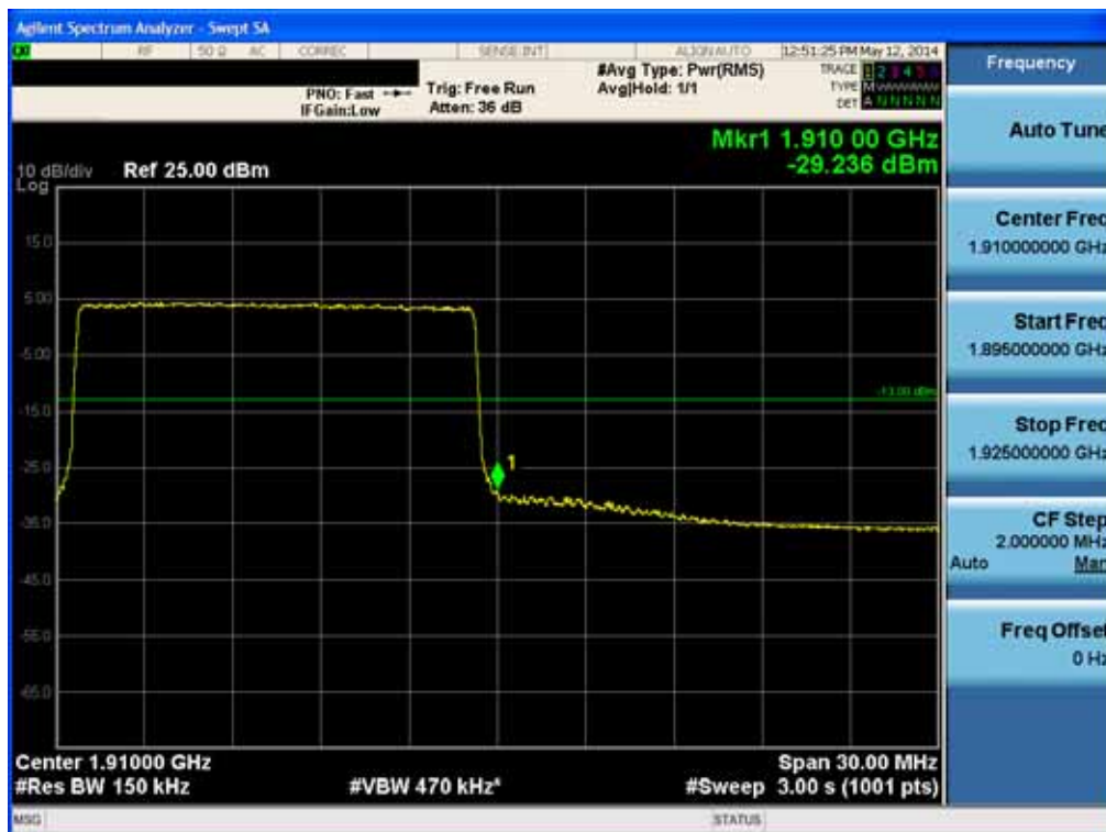
BAND 2. Upper Band Edge Plot (15M BW Ch.19125 QPSK RB 75) -2
