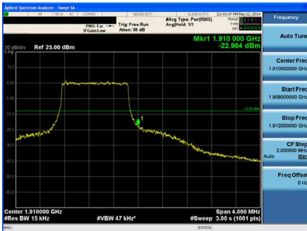
BAND 2. Upper Band Edge Plot (1.4M BW Ch.19193 QPSK RB 5) -2
