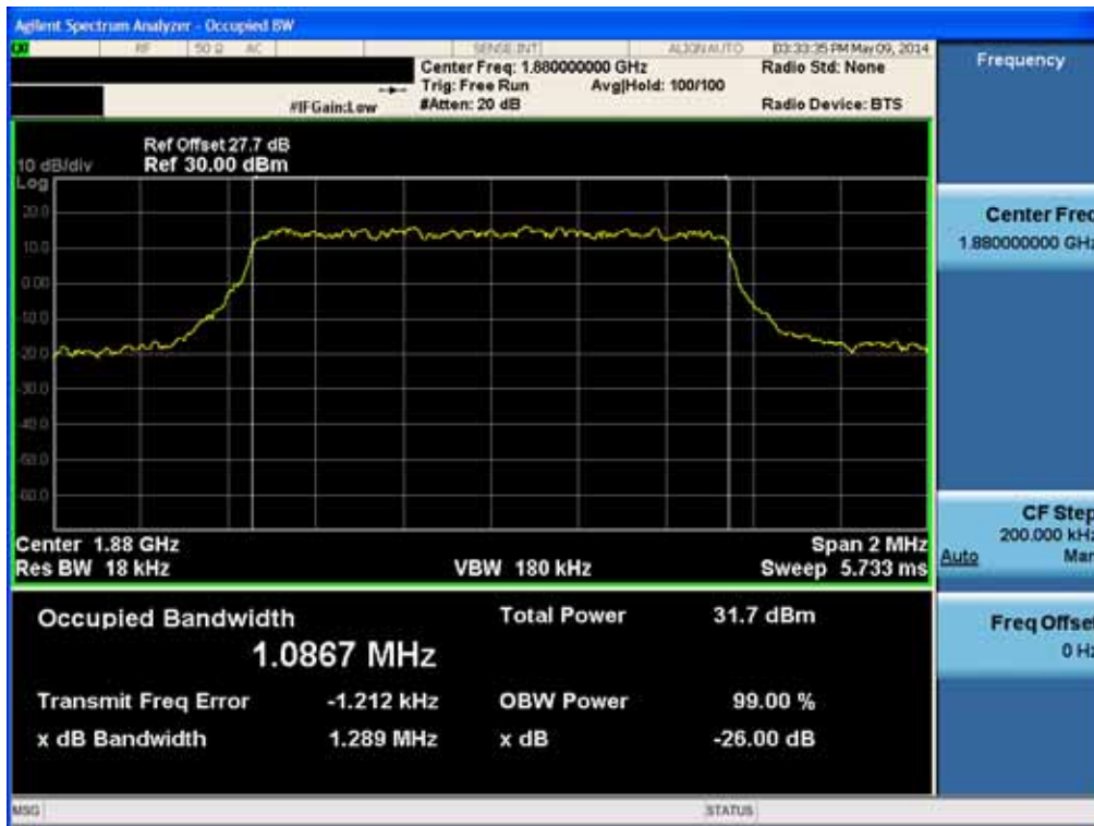
BAND 2. Occupied Bandwidth Plot (1.4M BW Ch.18900 QPSK RB 6_0)
