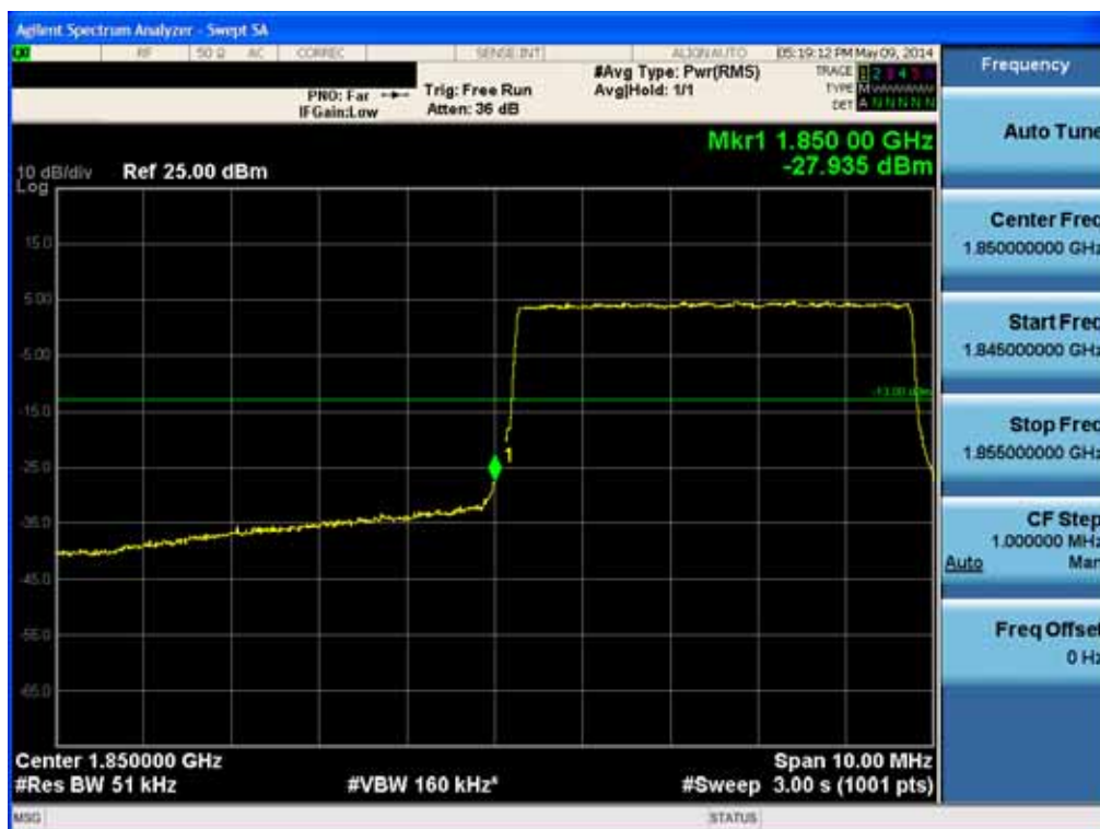
BAND 2. Lower Band Edge Plot (5M BW Ch.18625 QPSK RB 25) -2
