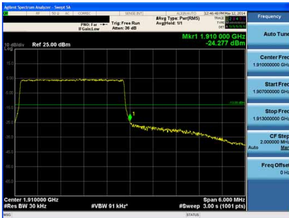
BAND 2. Upper Band Edge Plot (3M BW Ch.19185 QPSK RB 15) -2
