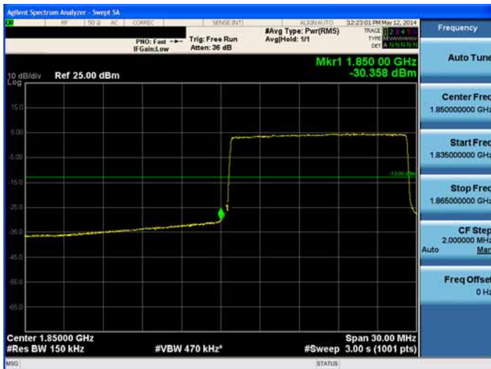
BAND 2. Lower Band Edge Plot (15M BW Ch.18675 QPSK RB 75) -2
