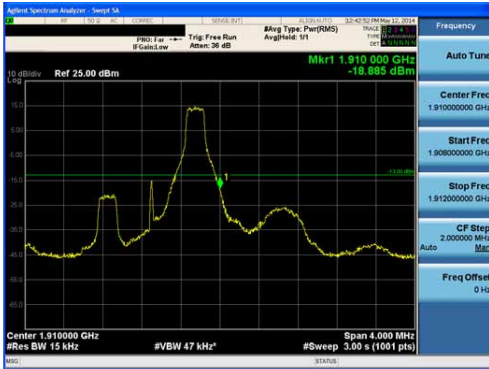
BAND 2. Upper Band Edge Plot (1.4M BW Ch.19193 QPSK RB 1, Offset 5) -1
