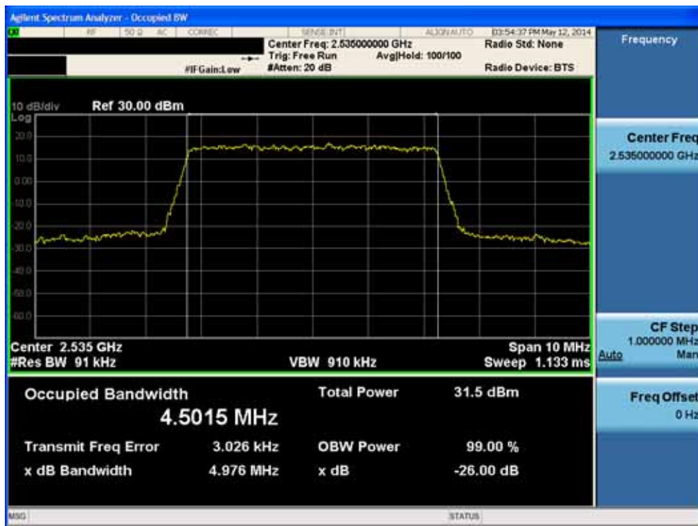
Occupied Bandwidth Plot (5MHz Ch.21100 QPSK RB 25)
