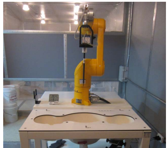
Figure 2.2 DASY5 Test System
