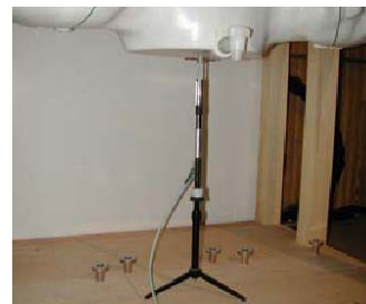
Figure 11.1 Dipole Verification Test Setup Diagram & Photo
