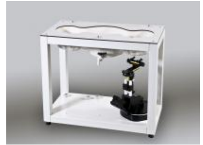
Figure 3.6 SAM Twin Phantom
