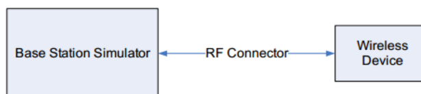
Figure 10.1 Power Measurement Setup
