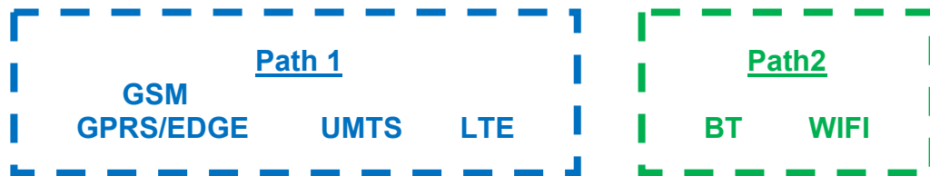
Figure 1-3 Simultaneous Transmission Paths
