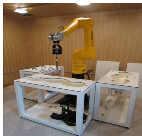
Figure 4.1 DASY5 Test System
