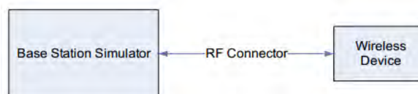
Figure 10.1 Power Measurement Setup
