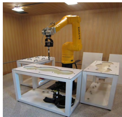
Figure 4.1 DASY5 Test System
