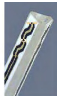
Figure 3.3 Probe Thick-Film Technique
