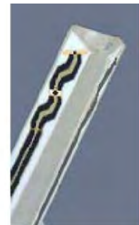
Figure 3.3 Probe Thick-Film Technique
