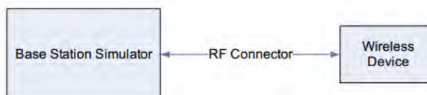
Figure 10.1 Power Measurement Setup
