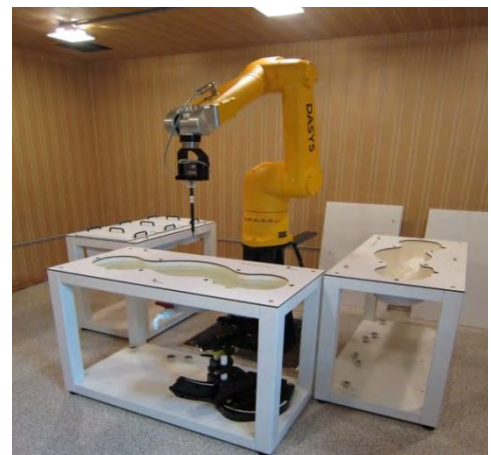
Figure 4.1 DASY5 Test System
