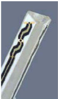
Figure 3.3 Probe Thick-Film Technique
