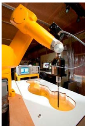
Figure 4-1 SAR Measurement System
