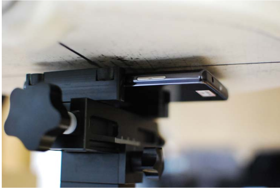
SAR Test Setup Photo 5: Back at 1.0 cm
