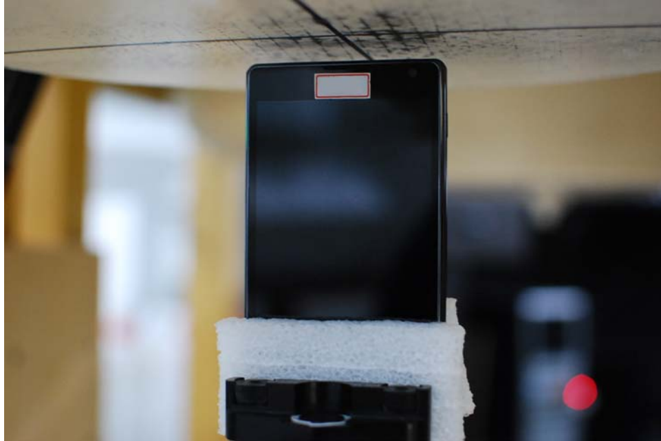
SAR Test Setup Photo 7: Top at 1.0 cm
