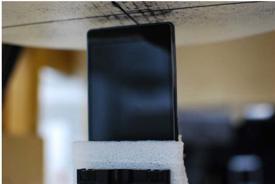
SAR Test Setup Photo 8: Bottom at 1.0 cm
