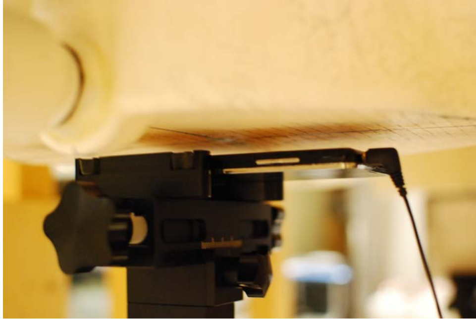
SAR Test Setup Photo 11: Body-Worn at 1.0 cm
