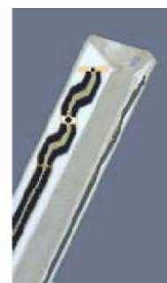
Figure 3.3 Probe Thick-Film Technique
