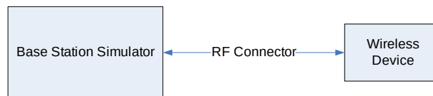
Figure 9-2 Power Measurement Setup
