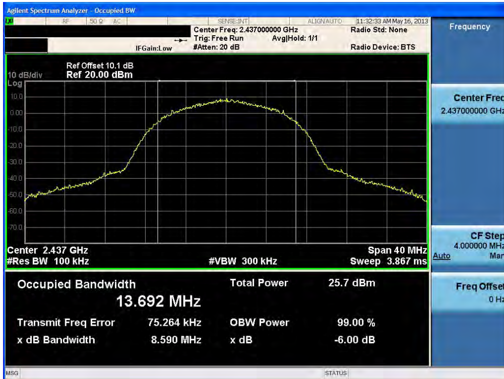
6dB Bandwidth plot (802.11b-CH 6)
