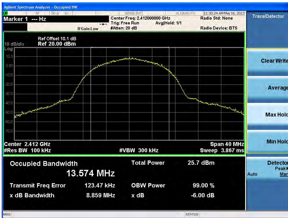
6dB Bandwidth plot (802.11b-CH 6)
