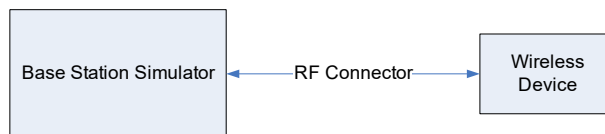
Figure 9-3 Power Measurement Setup
