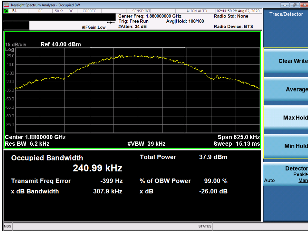
Plot 7-3. Occupied Bandwidth Plot (PCS GPRS Mode)
