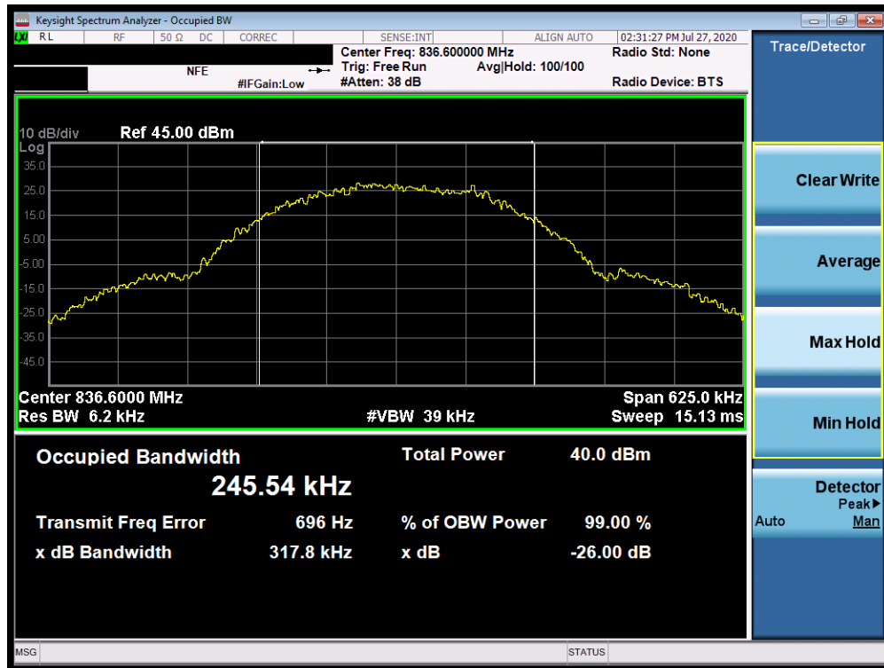
Plot 7-1. Occupied Bandwidth Plot (Cellular GPRS Mode)
