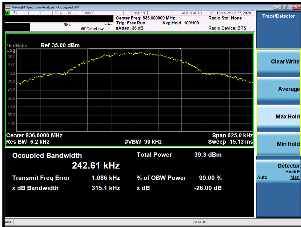
Plot 7-2. Occupied Bandwidth Plot (EDGE850 Mode)
