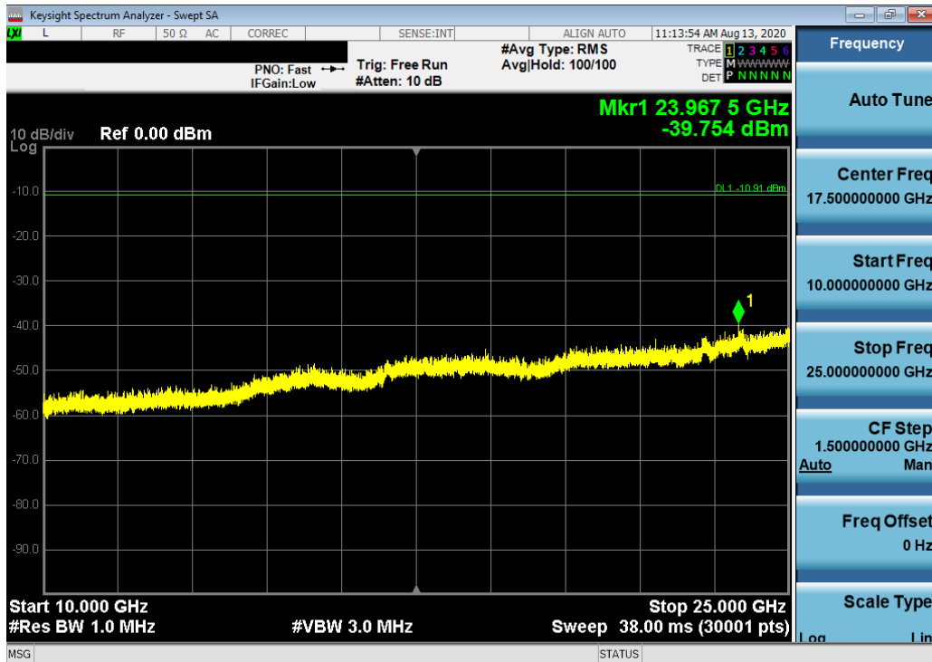
Plot 7-9. Conducted Spurious Plot (Bluetooth (LE), 1Mbps – Ch. 19)
