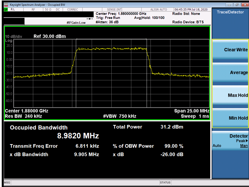
Plot 7-134. Occupied Bandwidth Plot (Band 25/2 - 10.0MHz 16-QAM - Full RB Configuration)
