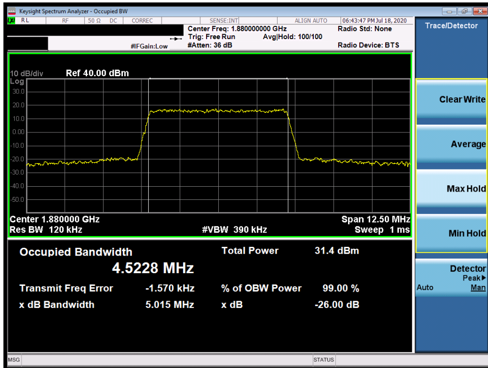
Plot 7-131. Occupied Bandwidth Plot (Band 25/2 - 5.0MHz 16-QAM - Full RB Configuration)
