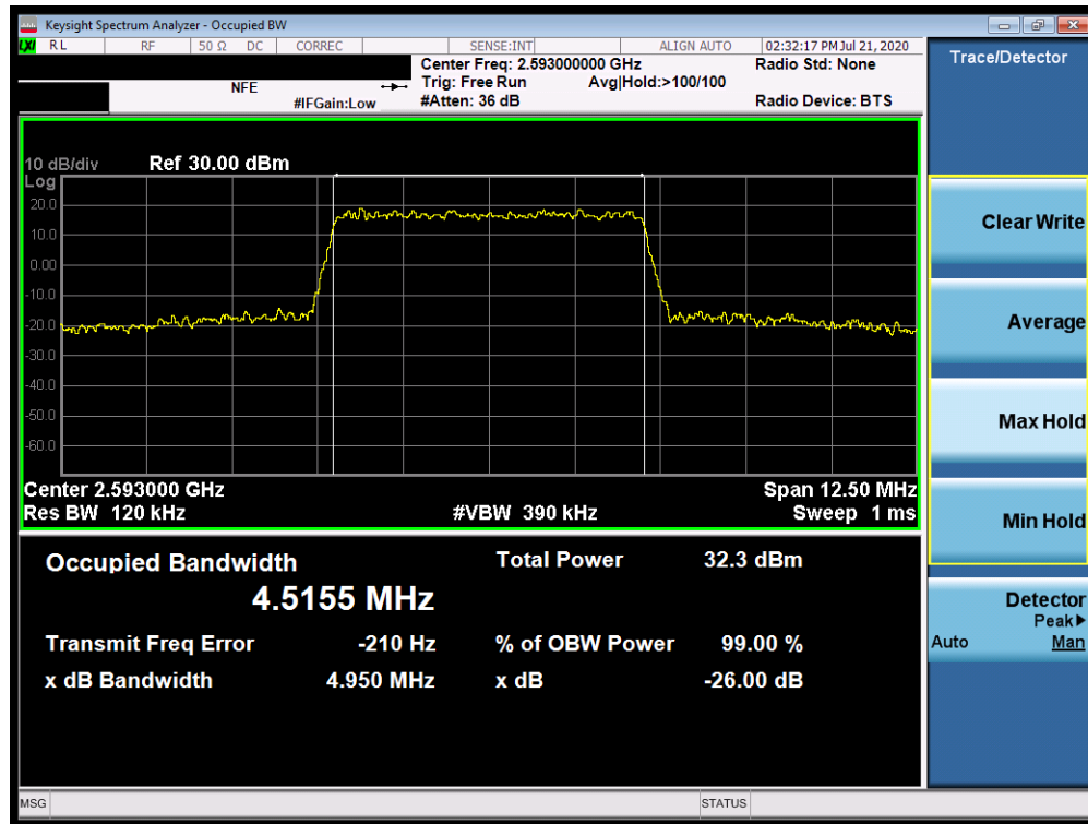
Plot 7-162. Occupied Bandwidth Plot (Band 41 – 5.0MHz QPSK - Full RB Configuration)
