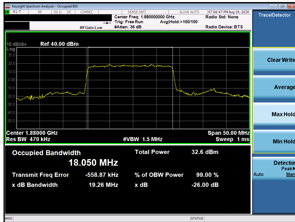
Plot 7-157. Occupied Bandwidth Plot (NR Band n25/2 - 20.0MHz DFT-s-OFDM BPSK - Full RB)
