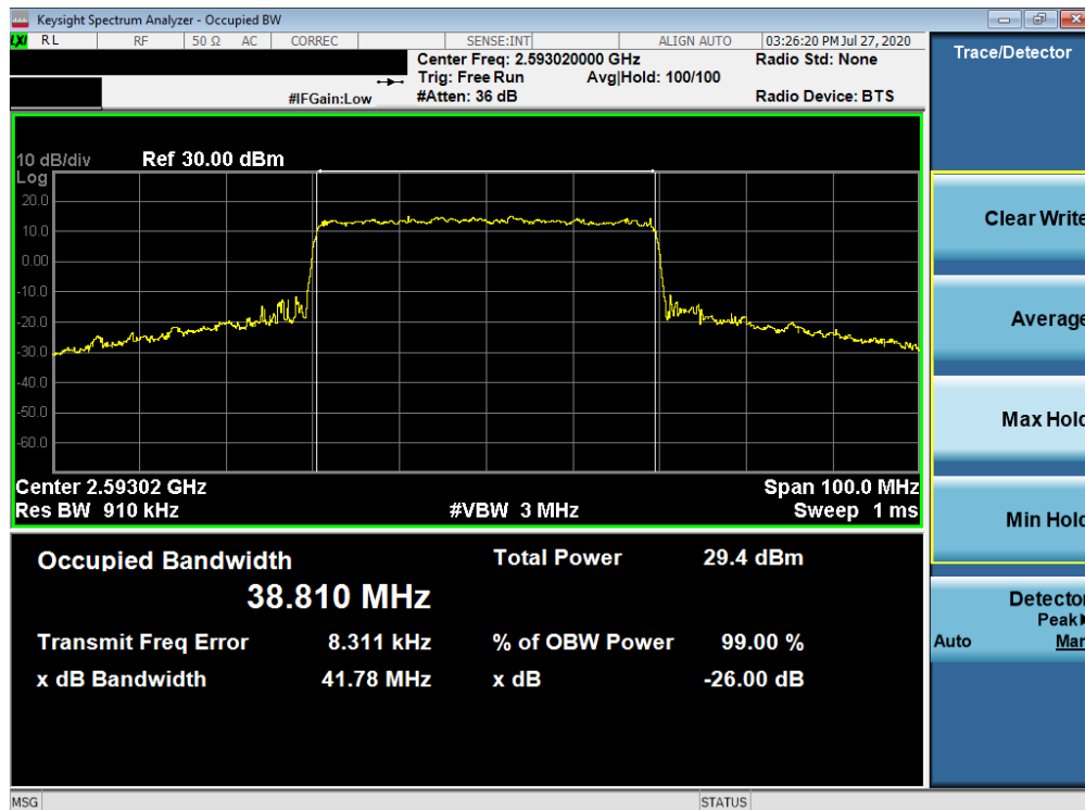
Plot 7-183. Occupied Bandwidth Plot (NR Band n41 - 40MHz CP-OFDM 256-QAM - Full RB)
