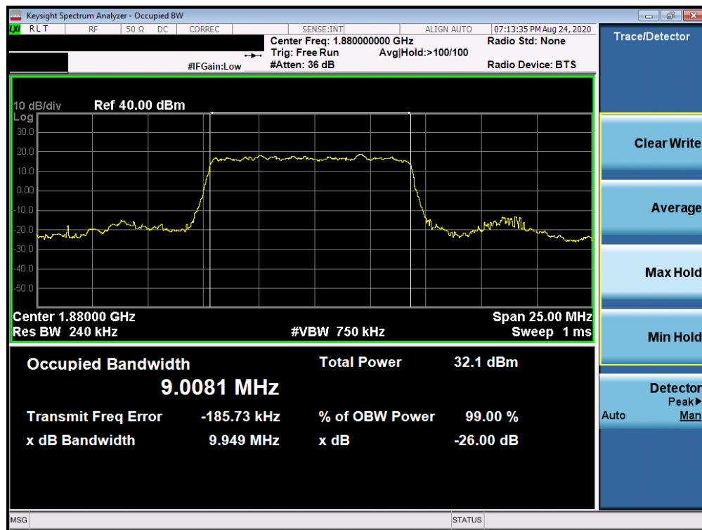
Plot 7-147. Occupied Bandwidth Plot (NR Band n25/2 - 10.0MHz DFT-s-OFDM BPSK - Full RB)
