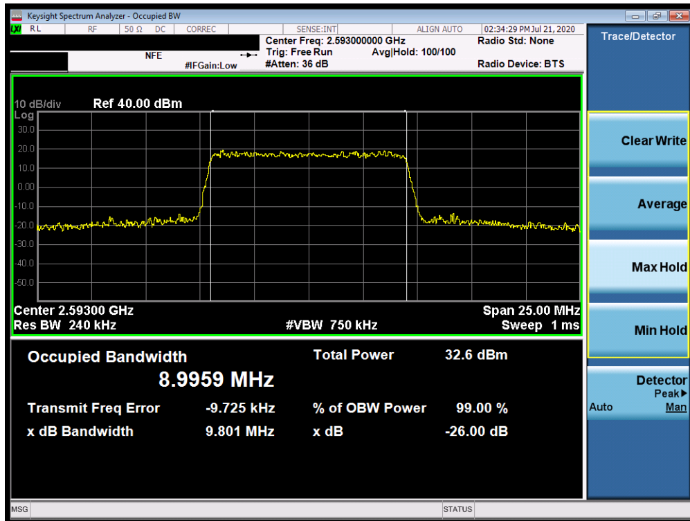
Plot 7-167. Occupied Bandwidth Plot (Band 41 - 10.0MHz 64-QAM - Full RB Configuration)
