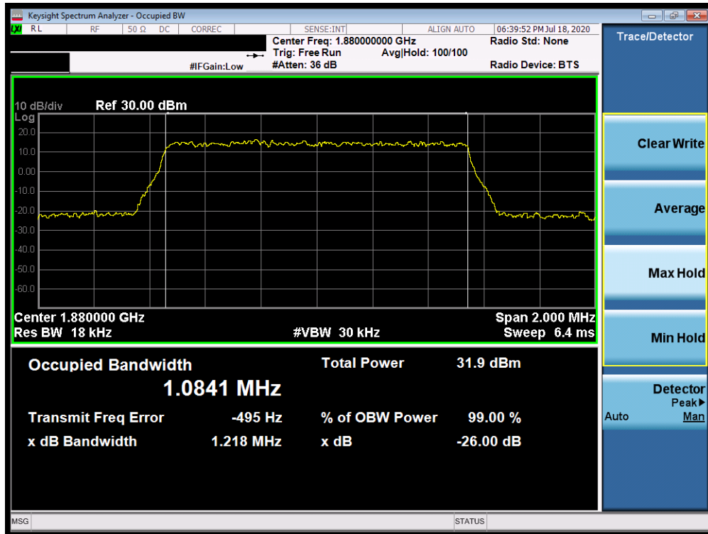
Plot 7-124. Occupied Bandwidth Plot (Band 25/2 - 1.4MHz QPSK - Full RB Configuration)
