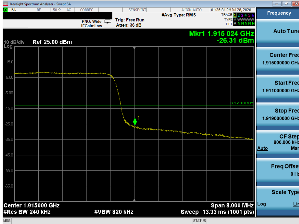
Plot 7-464. Upper Band Edge Plot (NR Band n25 – 10.0MHz - Full RB)
