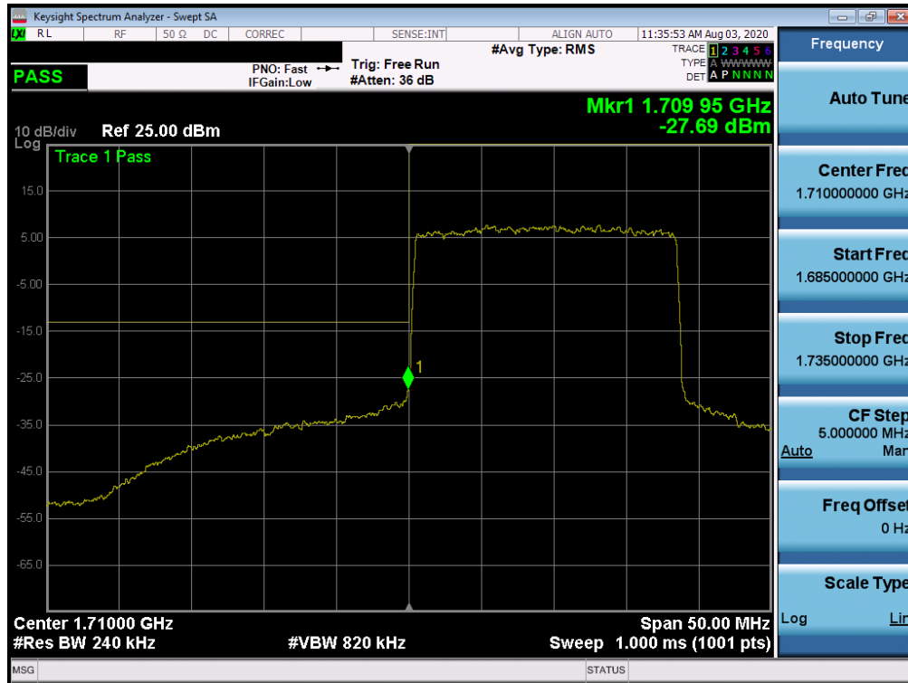
Plot 7-414. Lower Band Edge Plot (NR Band n66 – 20.0MHz - Full RB)
