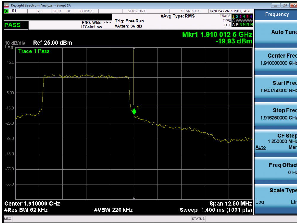
Plot 7-456. Upper Band Edge Plot (NR Band n2 – 5.0MHz - Full RB)
