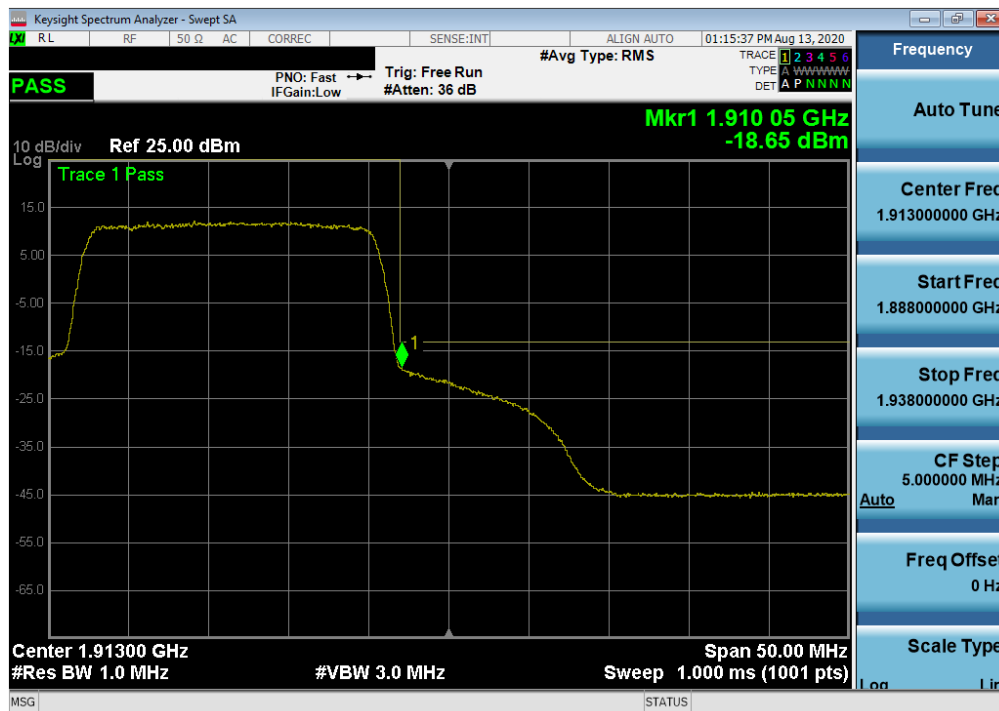
Plot 7-475. Upper Extended Band Edge Plot (NR Band n2 – 20.0MHz - Full RB)
