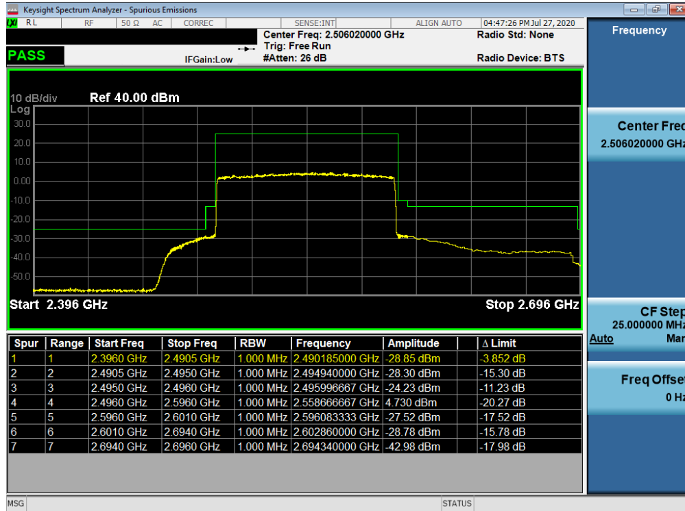
Plot 7-498. Lower ACP Plot (NR Band n41 - 100MHz CP-OFDM-QPSK - Full RB)
