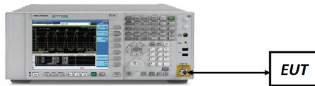
Figure 7-2. Test Instrument & Measurement Setup
