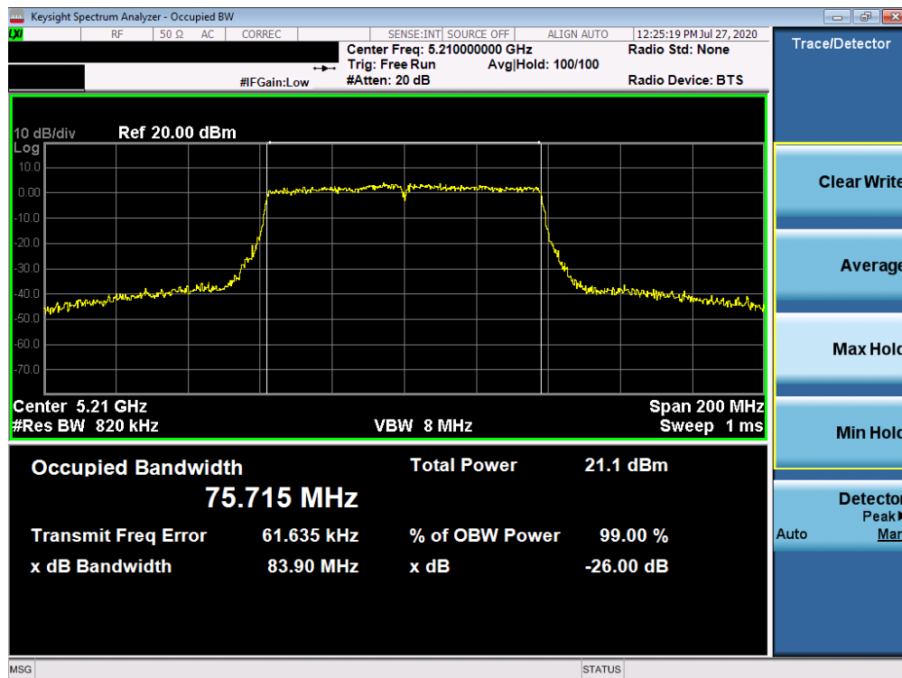
Plot 7-9. 26dB Bandwidth Plot SISO ANT1 (80MHz BW 802.11ac (UNII Band 1) – Ch. 42)
