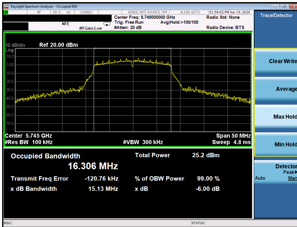
Plot 7-61. 6dB Bandwidth Plot SISO ANT1 (802.11a (UNII Band 3) – Ch. 149)
