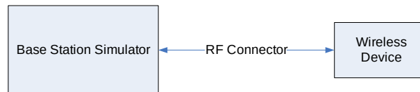
Figure 9-2 Power Measurement Setup
