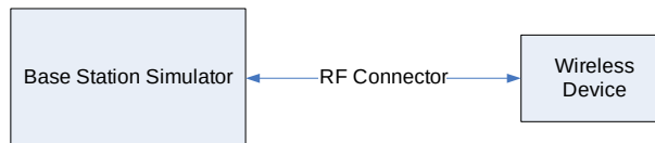
Figure 9-3 Power Measurement Setup
