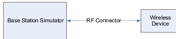
Figure 9-4 Power Measurement Setup
