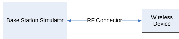
Figure 9-3 Power Measurement Setup
