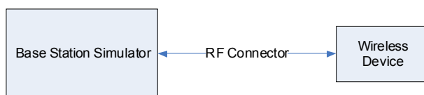
Figure 9-2 Power Measurement Setup
