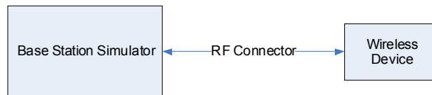
Figure 9-3 Power Measurement Setup
