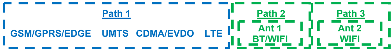
Figure 1-1 Simultaneous Transmission Paths
