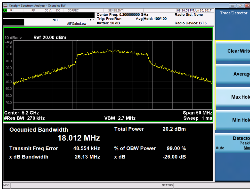
Plot 7-34. 26dB Bandwidth Plot (20MHz BW 802.11n (UNII Band 1) – Ch. 40)
