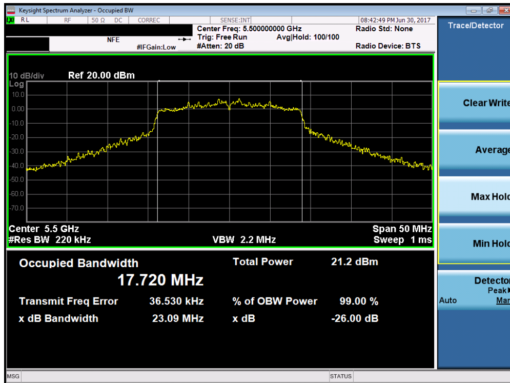
Plot 7-51. 26dB Bandwidth Plot (20MHz BW 802.11n (UNII Band 2C) – Ch. 100)
