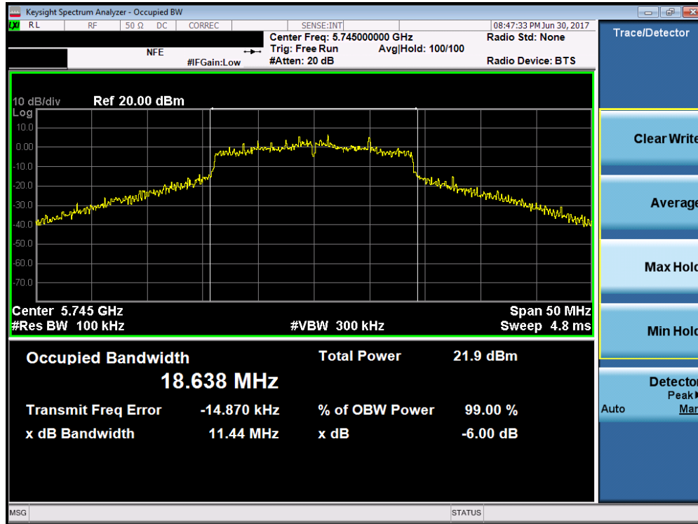
Plot 7-71. 6dB Bandwidth Plot (20MHz BW 802.11n (UNII Band 3) – Ch. 149)
