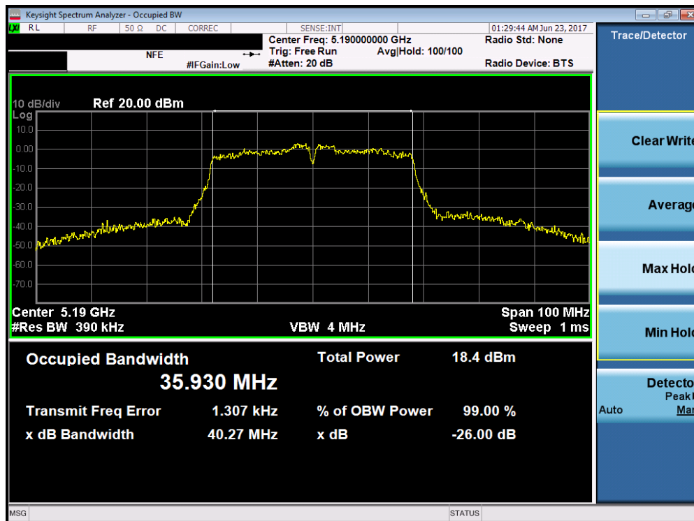
Plot 7-7. 26dB Bandwidth Plot (40MHz BW 802.11n (UNII Band 1) – Ch. 38)
