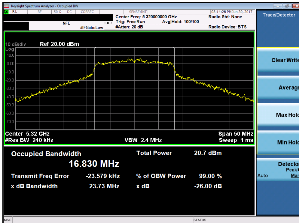
Plot 7-41. 26dB Bandwidth Plot (802.11a (UNII Band 2A) – Ch. 64)
