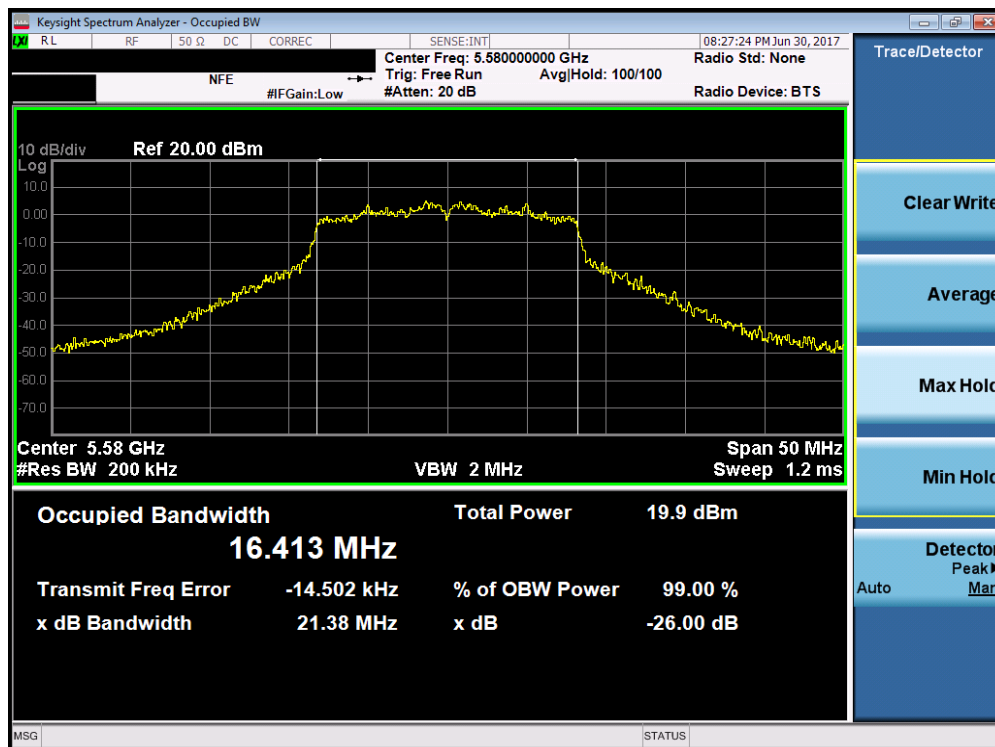
Plot 7-49. 26dB Bandwidth Plot (802.11a (UNII Band 2C) – Ch. 116)
