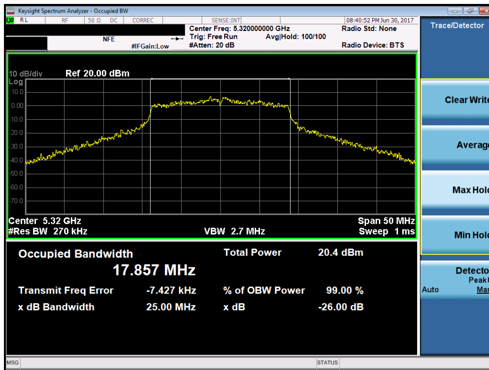
Plot 7-44. 26dB Bandwidth Plot (20MHz BW 802.11n (UNII Band 2A) – Ch. 64)
