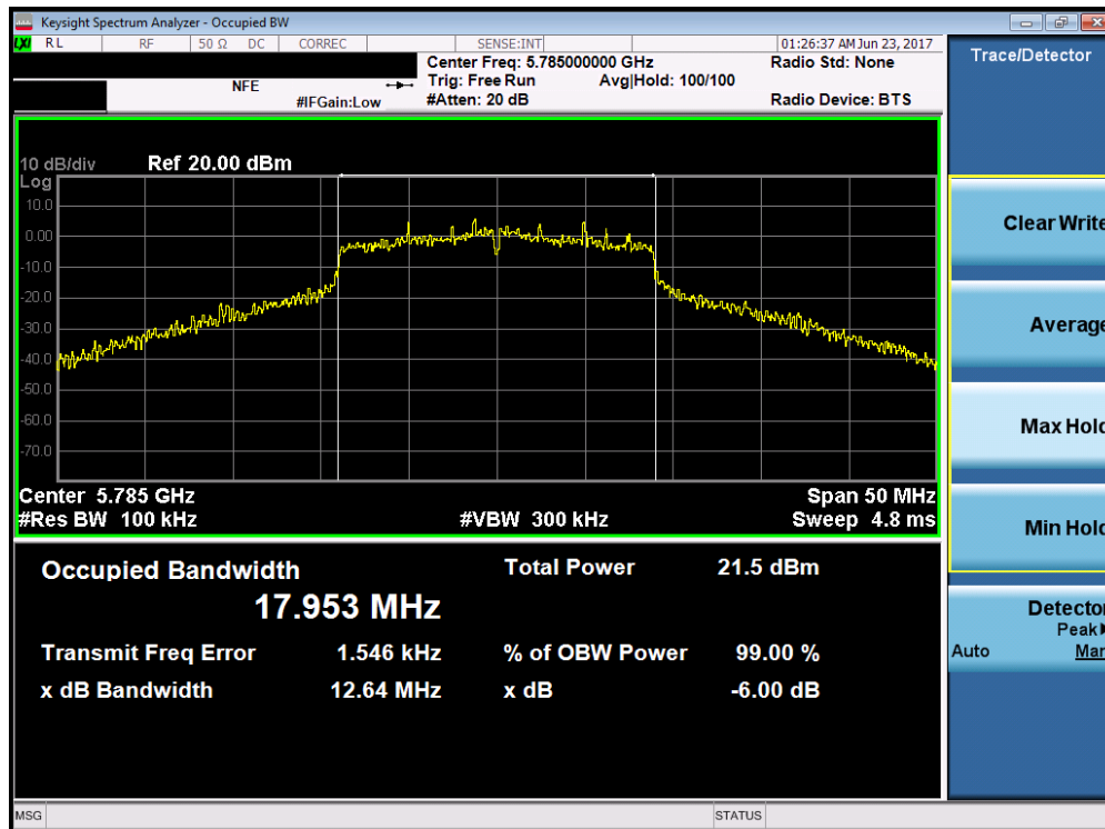
Plot 7-63. 6dB Bandwidth Plot (20MHz BW 802.11n (UNII Band 3) – Ch. 157)
