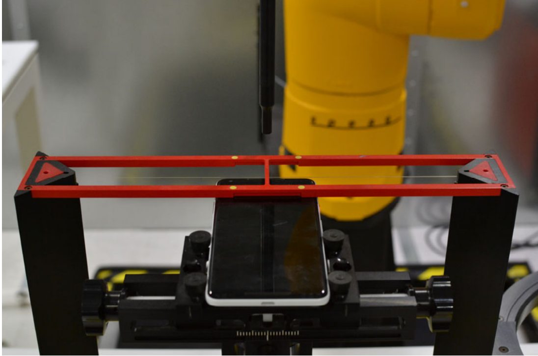
Figure 18-1 Ear Reference Point HAC Phantom Alignment
