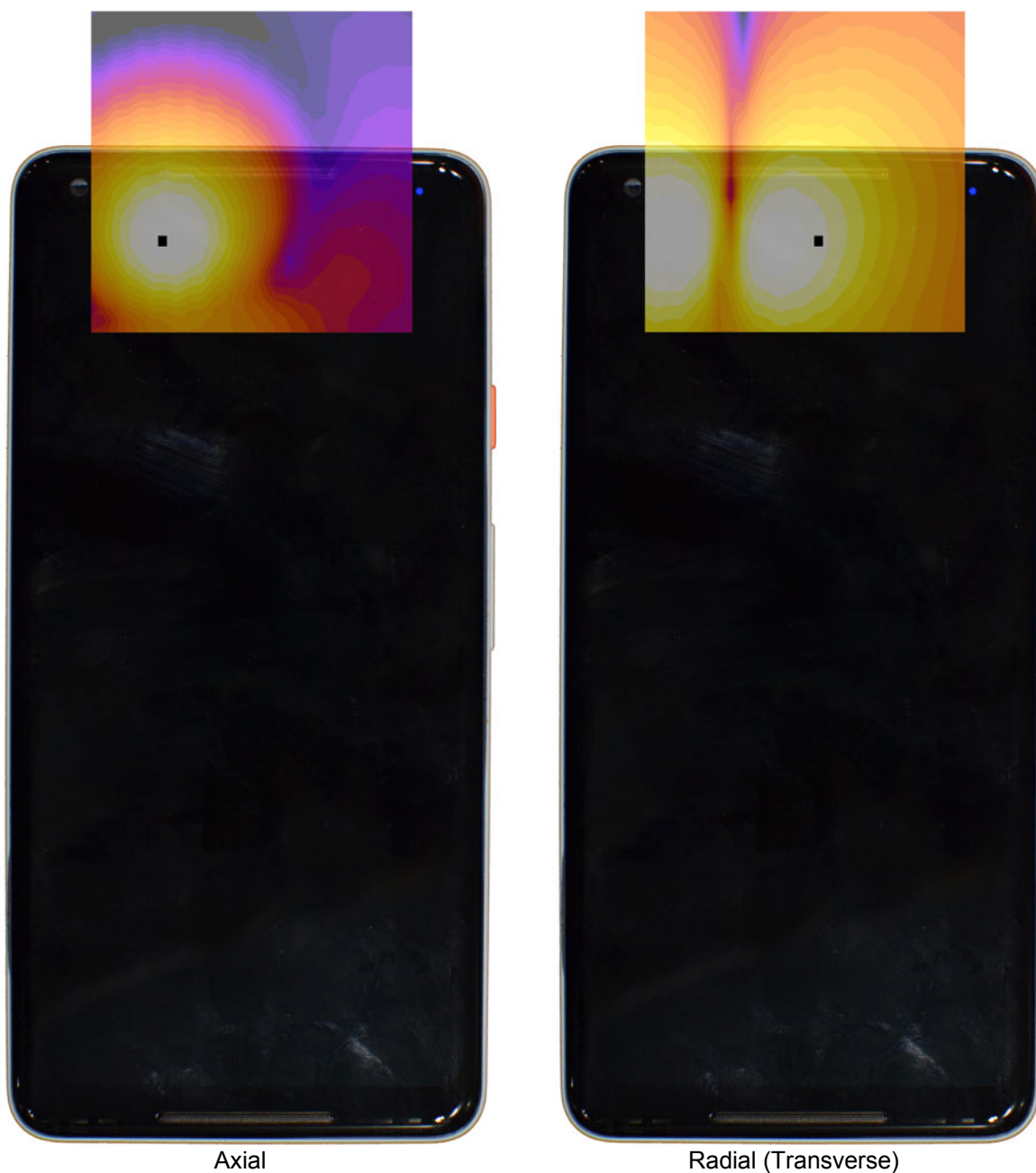
Figure 14-3 T-Coil Scan Overlay Magnetic Field Distributions
