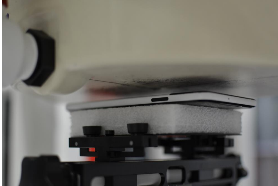
SAR Test Setup Photo 5: Back at 1.0 cm
