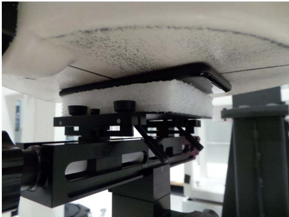
SAR Test Setup Photo 6: Back at 0.0 cm
