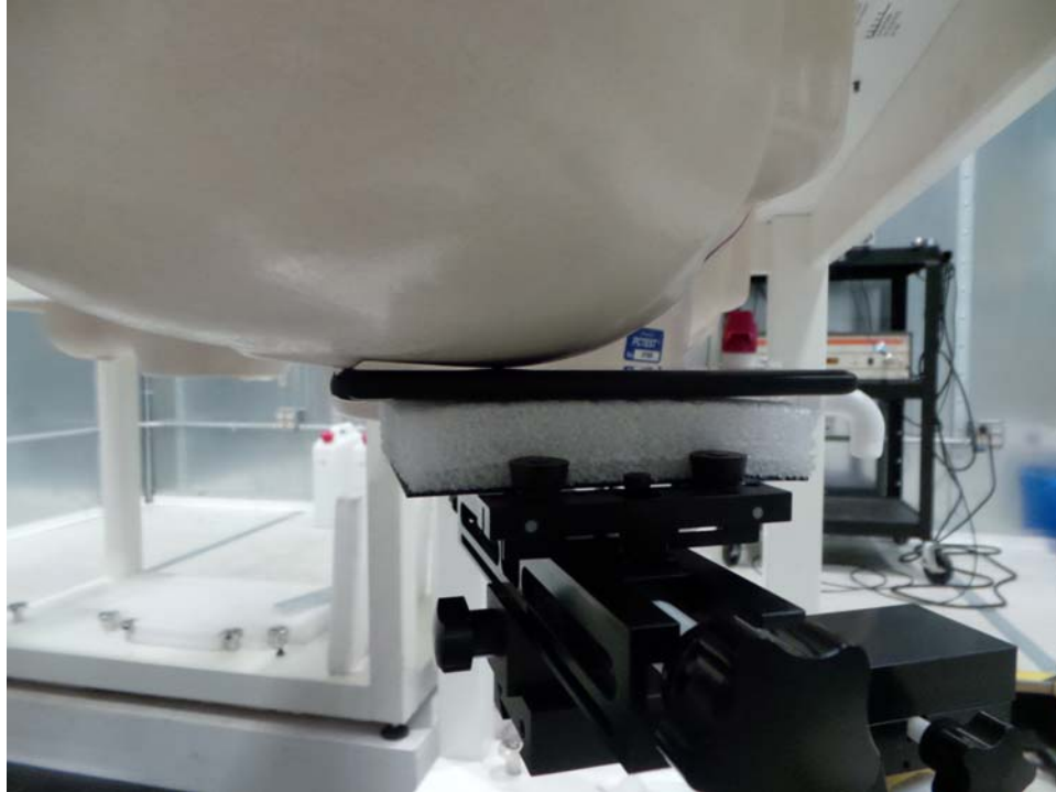
SAR Test Setup Photo 1: Right Cheek
