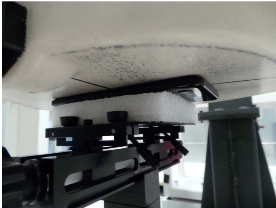
SAR Test Setup Photo 8: Front at 0.0 cm
