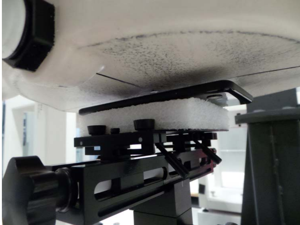
SAR Test Setup Photo 7: Front at 1.0 cm
