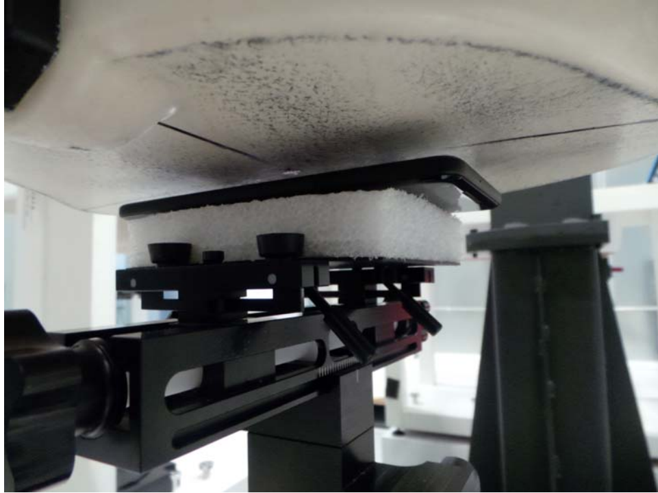
SAR Test Setup Photo 5: Back at 1.0 cm
