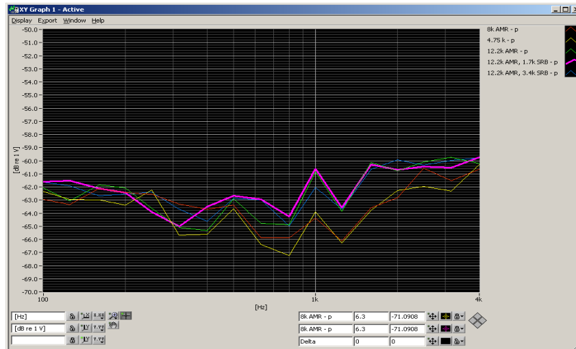
Figure 8-1 UMTS Audio Band Magnetic Noise
