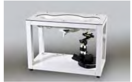
Figure 3.6 SAM Twin Phantom
