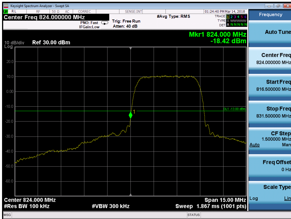
Plot 7-86. Band Edge Plot (Cellular WCDMA Mode - Low Channel)
