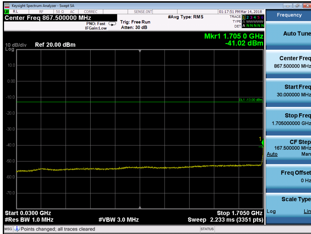
Plot 7-55. Conducted Spurious Plot (AWS WCDMA Mode - Low Channel)
