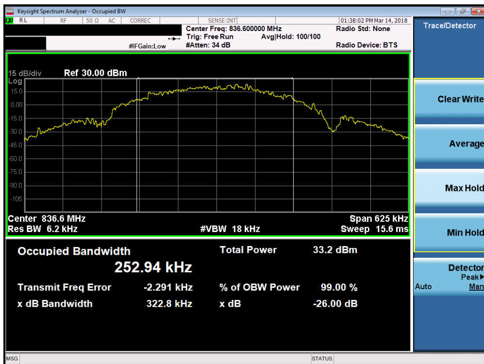
Plot 7-2. Occupied Bandwidth Plot (EDGE850 Mode)
