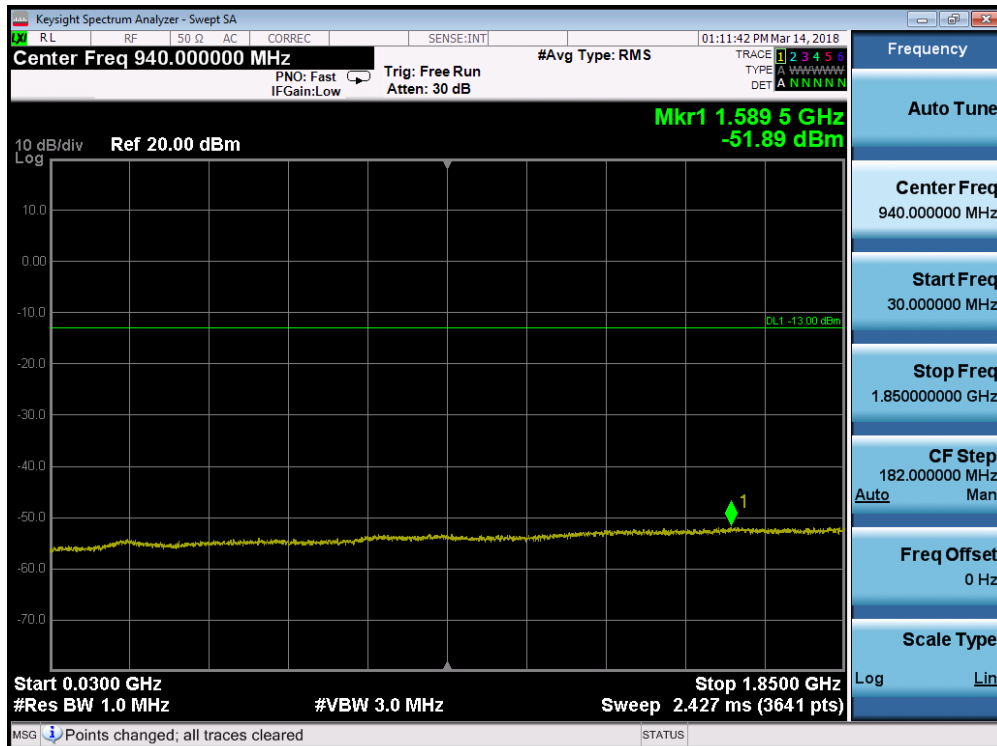
Plot 7-67. Conducted Spurious Plot (PCS WCDMA Mode - Mid Channel)
