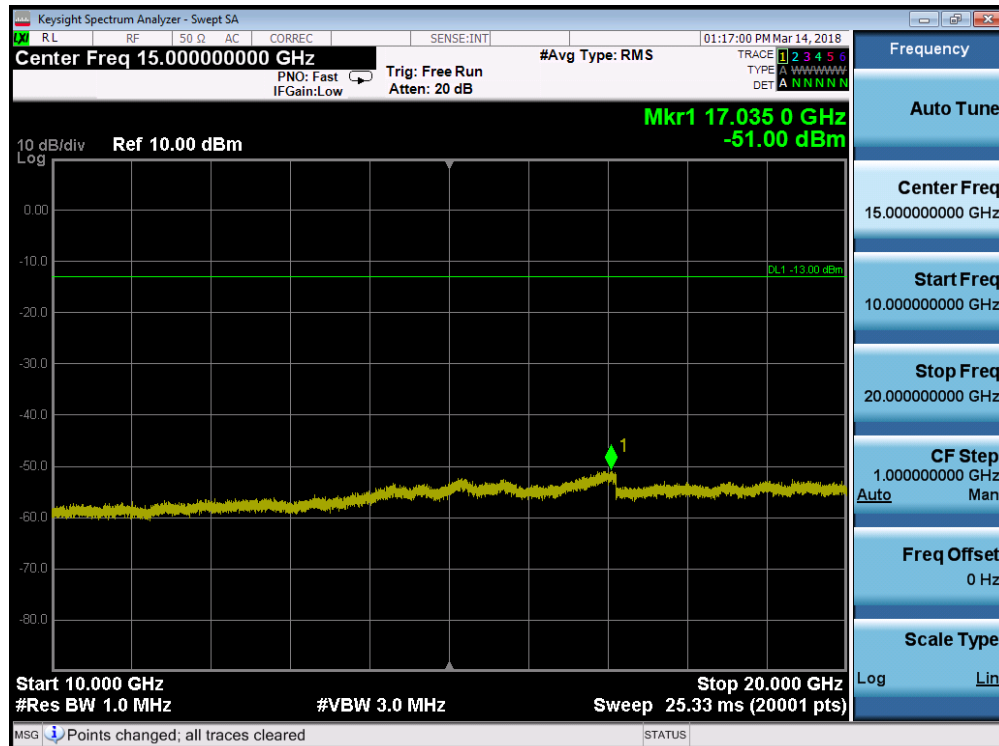
Plot 7-60. Conducted Spurious Plot (AWS WCDMA Mode - Mid Channel)
