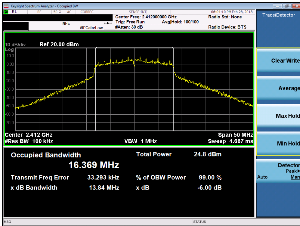
Plot 7-13. 6dB Bandwidth Plot (802.11g – Ch. 1)
