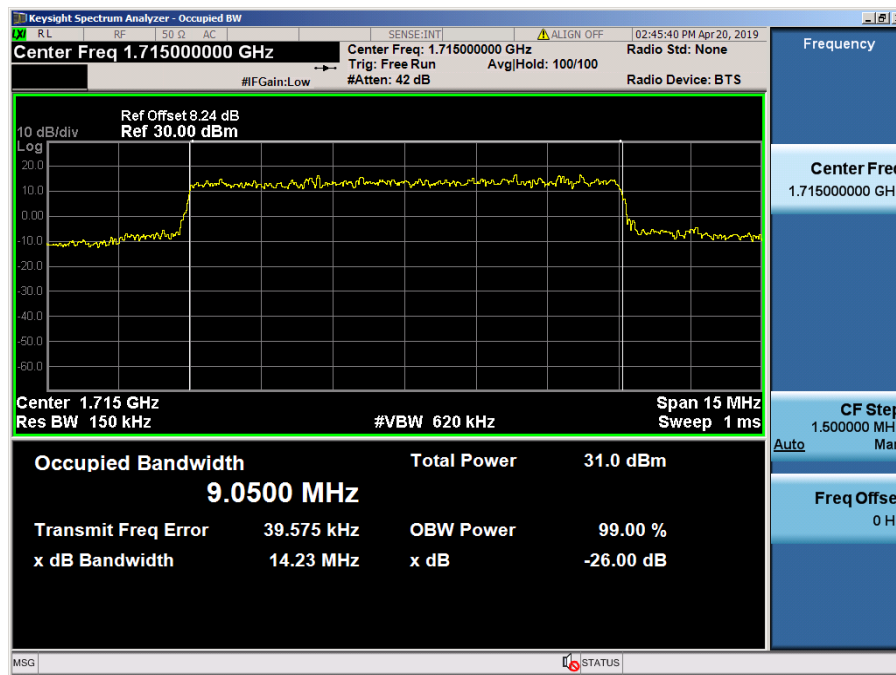
LTE Band 66, 4 / 10 MHz / QPSK - RB Size 50
