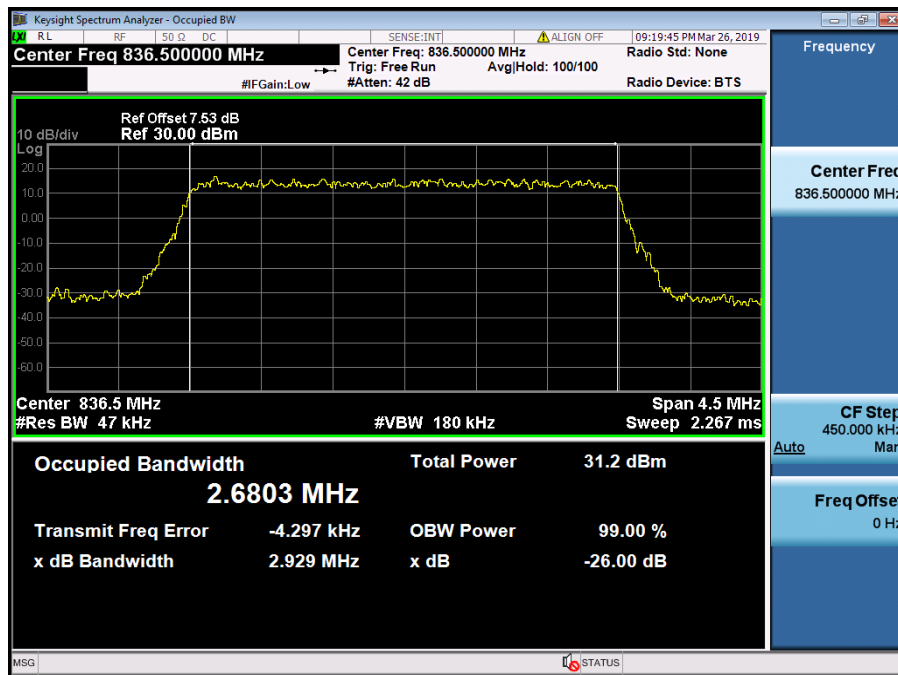
LTE Band 5, 26 / 3 MHz / QPSK - RB Size 15
