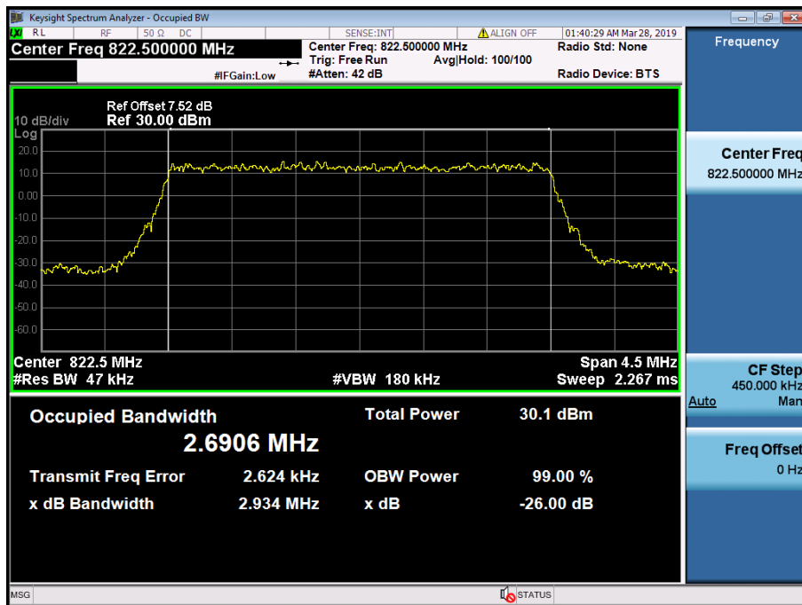
LTE Band 26 / 3 MHz / 16QAM - RB Size 15
