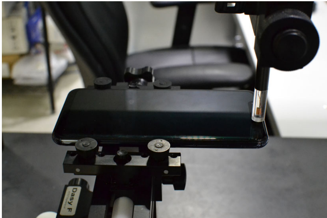
Figure 16-1 Test Setup for Wireless Device
