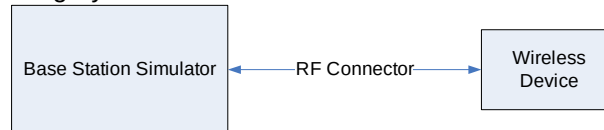
Figure 9-3 Power Measurement Setup
