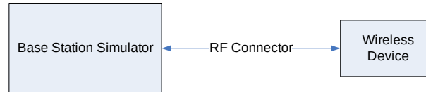
Figure 9-4 Power Measurement Setup
