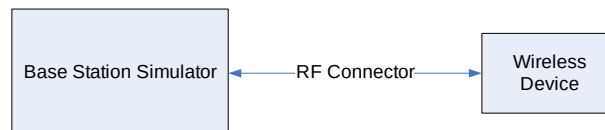
Figure 9-2 Power Measurement Setup
