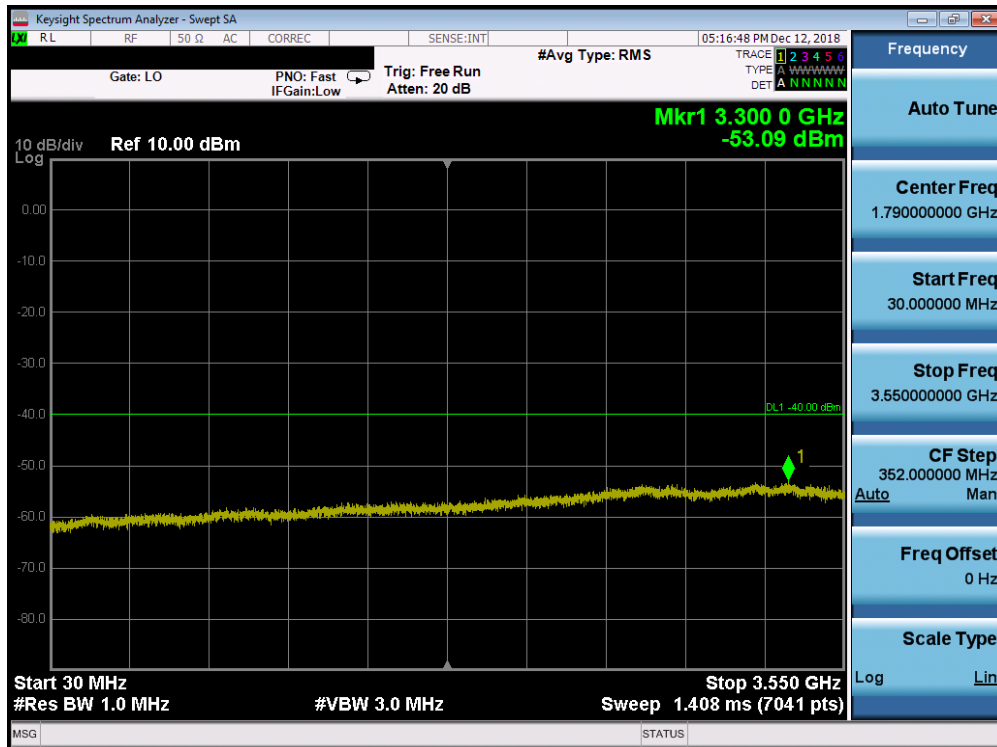
Plot 7-19. Conducted Spurious Plot (Band 48 - 20.0MHz QPSK - RB Size 1, RB Offset 0 - High Channel)
