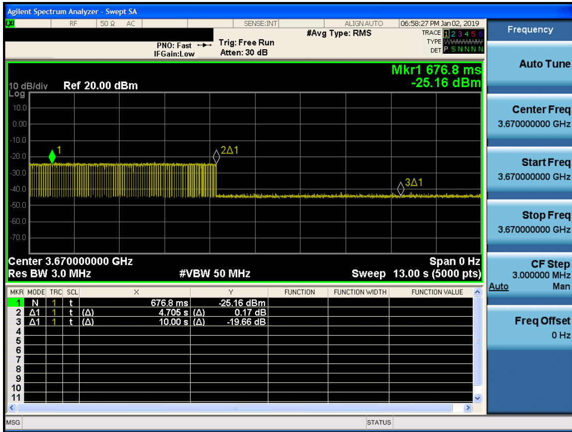
Plot 7-38. Run#2 End User Device Discontinues Operations within 10s
