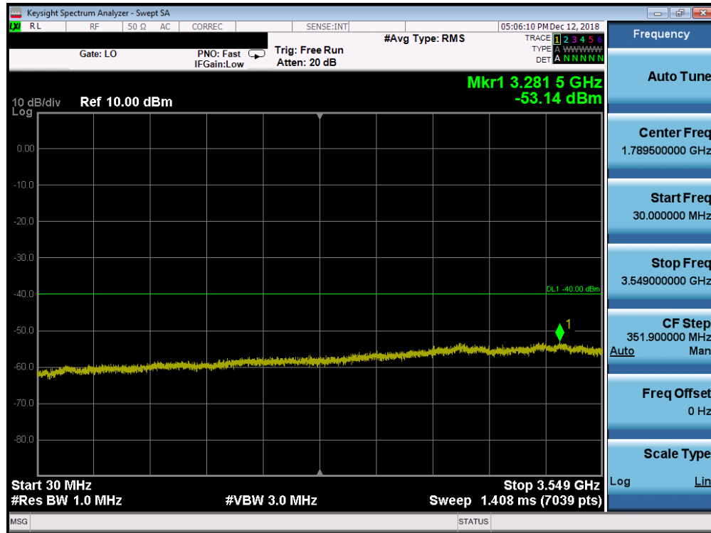
Plot 7-13. Conducted Spurious Plot (Band 48 - 20.0MHz QPSK - RB Size 1, RB Offset 0 - Low Channel)
