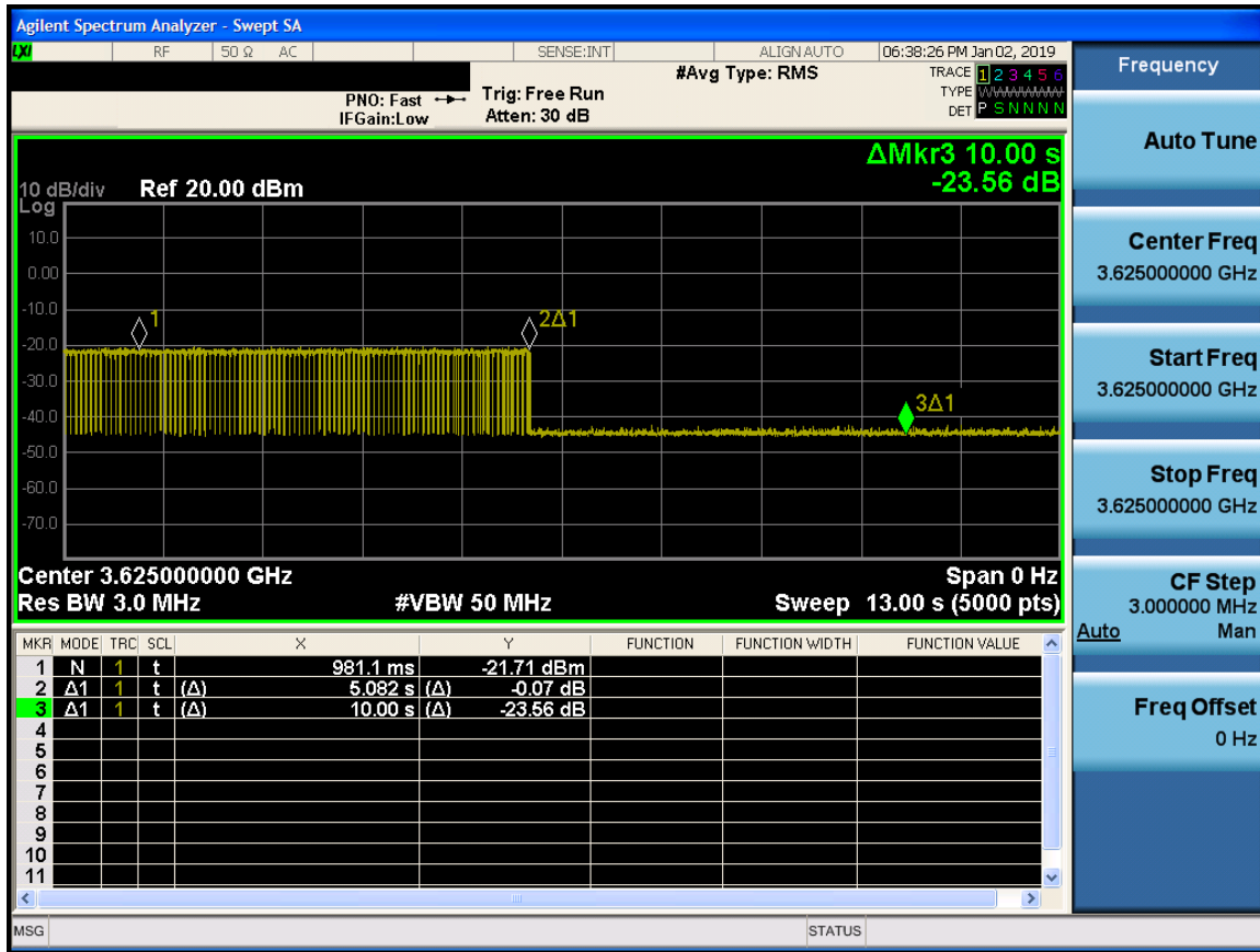
Plot 7-36. Run#1 End User Device Discontinues Operations within 10s
