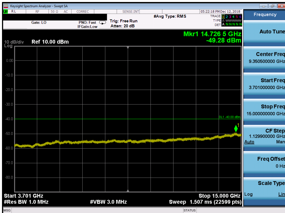
Plot 7-20. Conducted Spurious Plot (Band 48 - 20.0MHz QPSK - RB Size 1, RB Offset 0 - High Channel)
