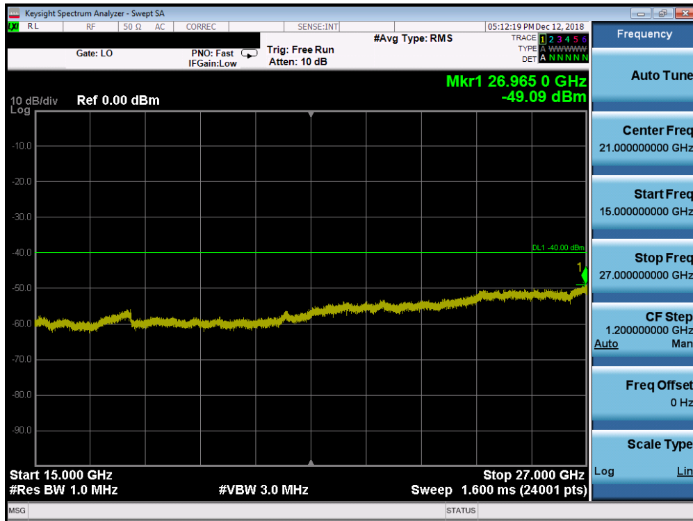
Plot 7-15. Conducted Spurious Plot (Band 48 - 20.0MHz QPSK - RB Size 1, RB Offset 0 - Low Channel)
