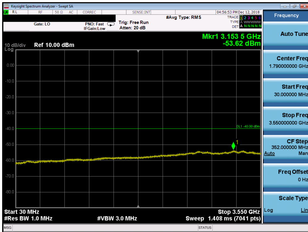
Plot 7-16. Conducted Spurious Plot (Band 48 - 20.0MHz QPSK - RB Size 1, RB Offset 0 - Mid Channel)
