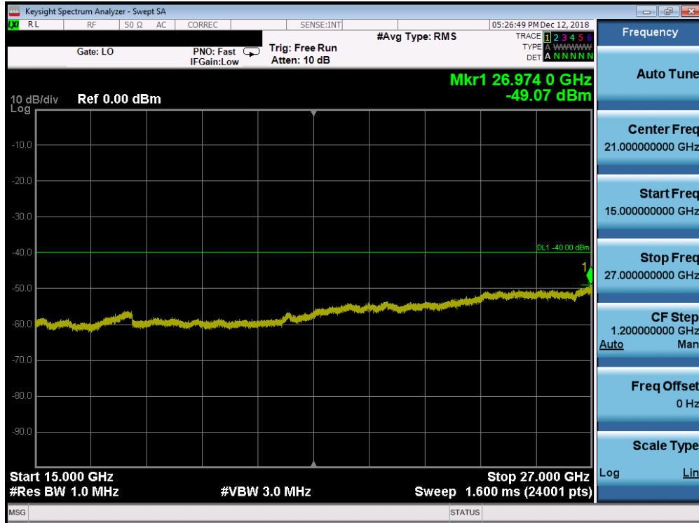
Plot 7-21. Conducted Spurious Plot (Band 48 - 20.0MHz QPSK - RB Size 1, RB Offset 0 - High Channel)
