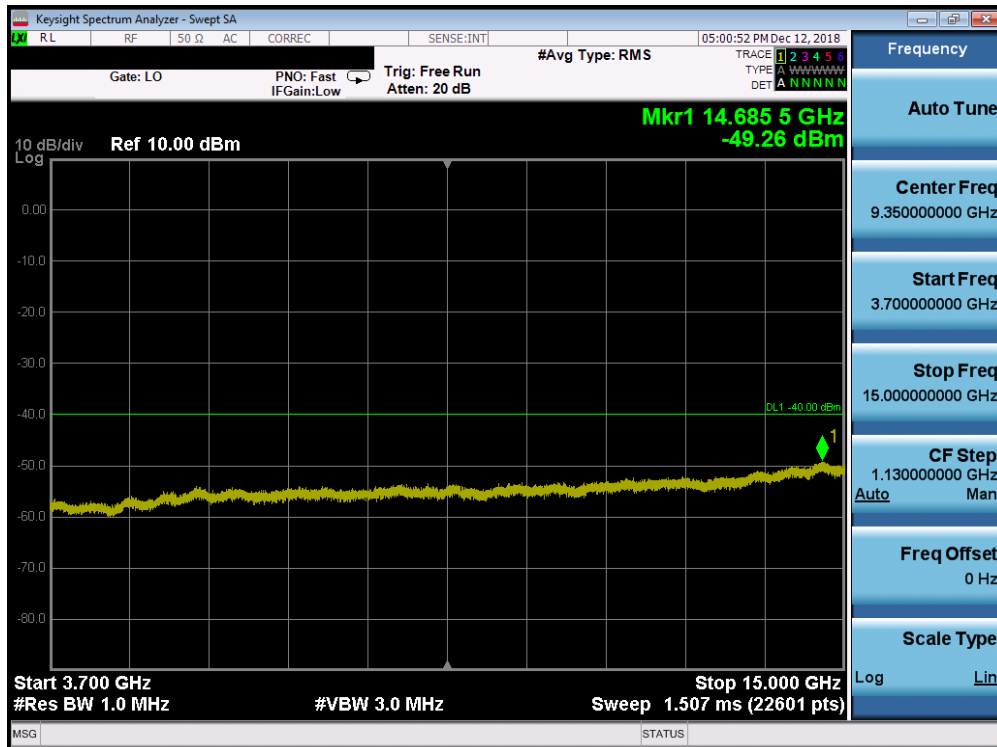
Plot 7-17. Conducted Spurious Plot (Band 48 - 20.0MHz QPSK - RB Size 1, RB Offset 0 - Mid Channel)
