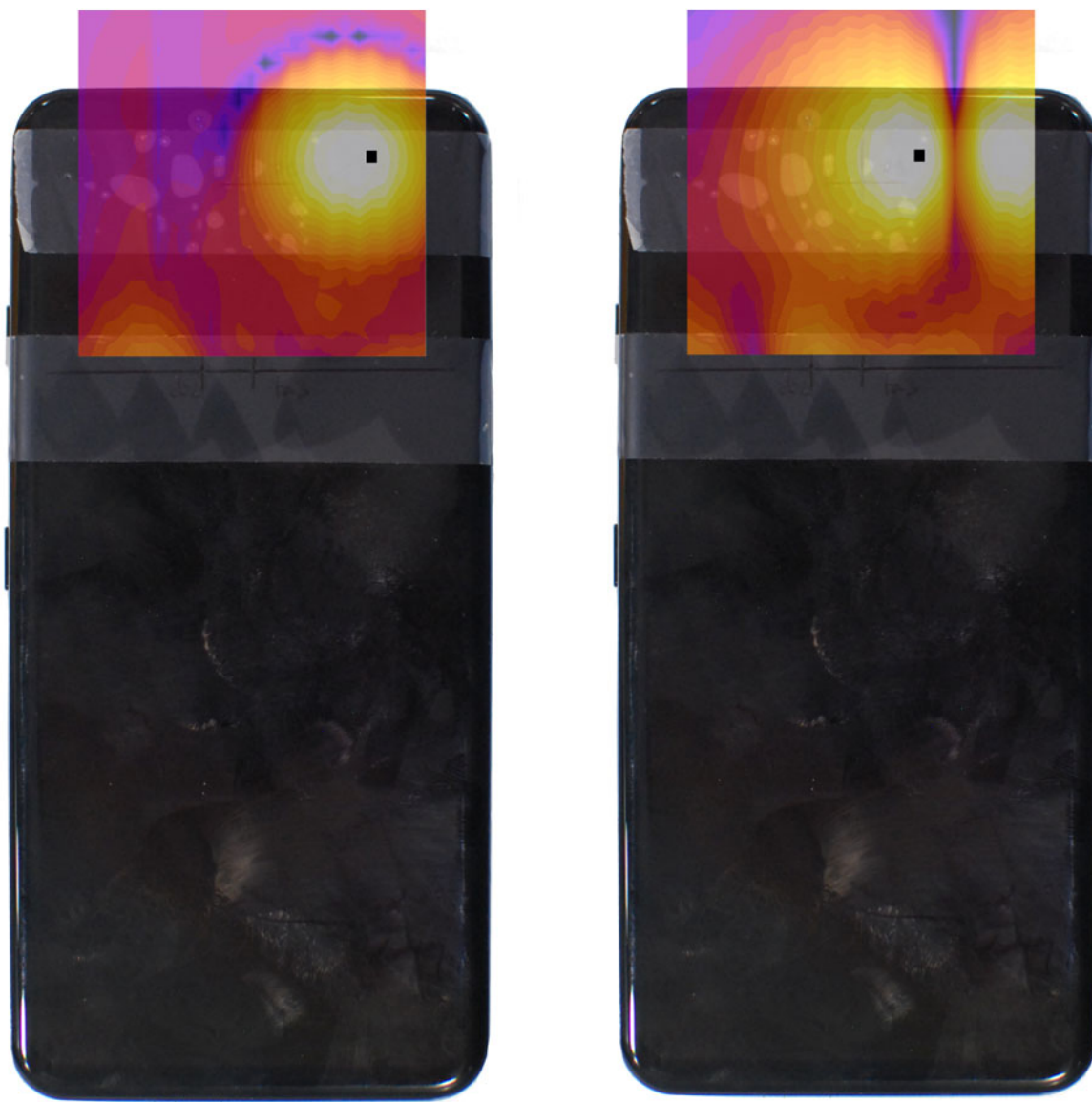
Figure 16-3 T-Coil Scan Overlay Magnetic Field Distributions
