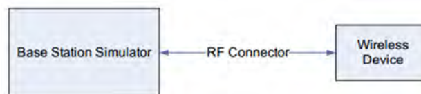
Figure 9.1 Power Measurement Setup
