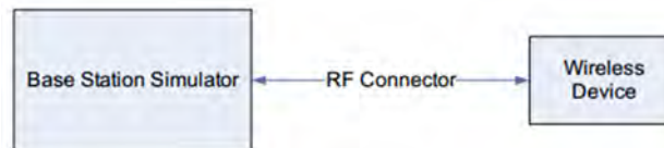
Figure 9.1 Power Measurement Setup
