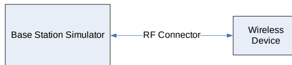
Figure 9-4 Power Measurement Setup
