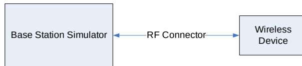
Figure 9-3 Power Measurement Setup
