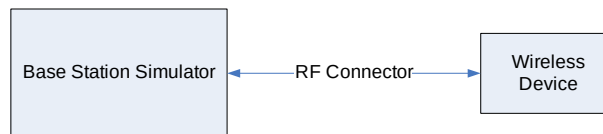
Figure 9-4 Power Measurement Setup
