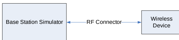
Figure 9-1 Power Measurement Setup
