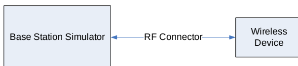
Figure 9-1 Power Measurement Setup
